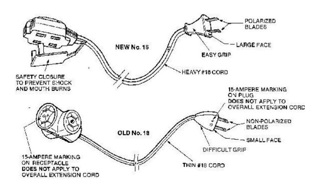
Overheating of the entire cord is usually caused by overloading (connecting appliances that need too many watts for the wire size of the cord). Many older extension cords made with small (No. 18 gauge) wire that can overheat at 15 or 20 amps are in use.
